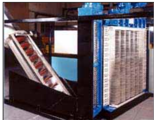
Screw Extraction Package Up to 13,900m 3 /h
