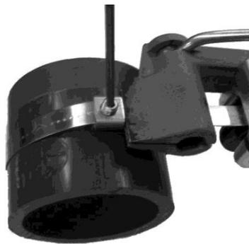
2. After tension is applied, insert set screw in Scru-Lokt buckle and tighten. To permit taking up Scru-Lokt clamp, or to re-use, a 3 inch (7.5 cm) stub should be left so that tool will be able to re-grip band later.
