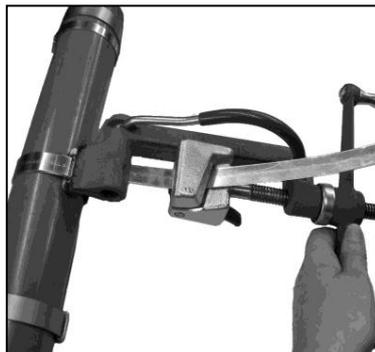
5. Roll tool over buckle, *backing off with tension handle throughout entire rolling operation.* Failure to back off with tension handle through-out entire course of roll-over may result in breaking of band. There is no loss of tension as band released is used up in the bend.
