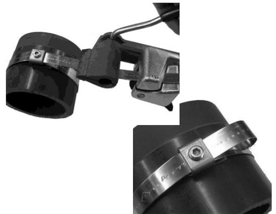
3. Where stub of band is left for Scru-Lokt clamp, it may be folded under as shown.
