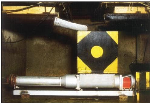
◀ A custom-built W082 is speeding up waste disposal at a Scottish tannery. Previously the 'fleshings' were shovelled manually from the processing area to a skip, this method was highly labour intensive. The cast iron W range pump with large auger and hopper were specially modified in order to handle this difficult material. The fleshings waste is gravity fed into the hopper, then pumped at 5.5m<sup>3</sup>/h at a pressure of 3 bar, along 30m of pipe direct to an outside skip for disposal.
