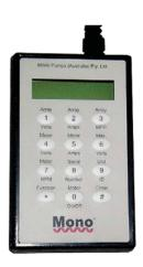
The display unit can be powered directly from the STC or from its internal 9 volt battery. If the STC is powered, the Display unit takes power from the STC (i.e. it will operate even if the Display unit battery is flat.) If the STC is not connected to an array or the STC battery is flat, the display unit can power the STC via the Display unit's internal battery.
