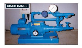
CB pump unit used for dosing various grades of polyelectrolyte in the paper industry at flows up to 500 l/h and pressures up to 2.5 bar. The customer requested specific drive characteristics to achieve a robust and reliable pump unit. To date, this range of pumps has proved to be very successful for this customer.
