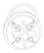
The SMC will only operate when pins 3 and 4 of the float switch are connected. The blanking plug contains a link wire to connect these two pins. External switches can be wired into the float switch to remotely start and stop the pump.
