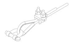
Connect the stainless steel safety cable to the pump as shown below. (Note the motor is not shown for clarity.)
