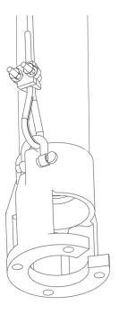
The other end of the safety cable will be connected to the bore cap when the pump has been installed.
