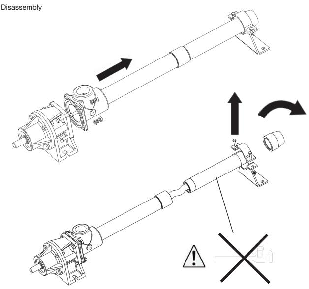
Do Not Use pipe wrench on Stator Barrel, as compression may effect pump performance
