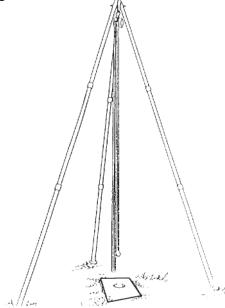
Pre-Assembly of the Drive Shaft Lengths.
