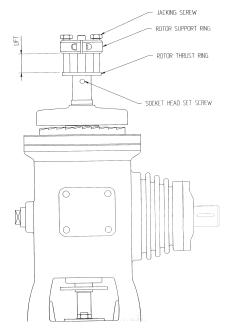
12. If the required height for setting the pump has been achieved, fit and tighten the socket set screws into the drive head main shaft, so as to lock the final connecting shaft to the main shaft.
