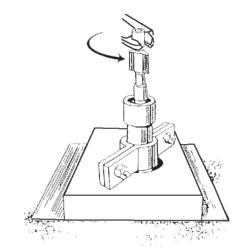
The short piece of column is used last. This piece enables easier connection of the drive head due to having the end of the column closer to the ground. The final column assembly is shown below.
