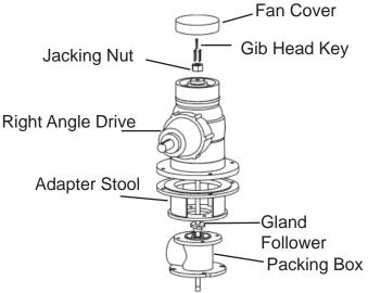
3. Before installing the RD-F30A drive head to the pump column it is important to make sure oil flows into the input shaft housing. To do this fill the main gear case to the correct level and tip the drive head forward until the input drive shaft hits the ground. The recommended Oils for this drive head are as below. To fill the drive head this requires approximately 1.5 litres of oil.
