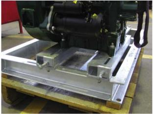
The photo graph below shows a typical right angle drive set up (guard removed for clarity). Note: Guard must be installed prior to operation.
