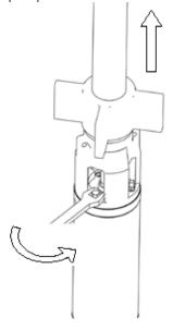
Pull the pump off the rotating assembly being careful to pull in a straight line to prevent damage to the flexishaft coating.
