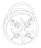
The SMC will only operate when pins 3 and 4 of the float switch are connected. The blanking plug contains a link wire to connect these two pins. External switches can be wired into the float switch to remotely start and stop the pump.
