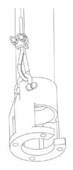
The other end of the safety cable will be connected to the bore cap when the pump has been installed.
