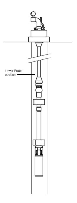
As an initial setting the top probe should be positioned about 1 metre above the bottom probe. It is not necessary to separate the probes by a large distance as it is with some AC pumping systems. (In AC systems the probe separation is used to control the number of pump starts per hour because more than 20 starts per hour can cause the motor to overheat). The SB3 system will not be damaged by repeated starts so large separations are not required.
