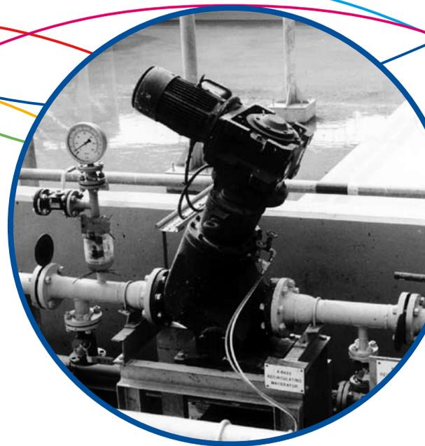
Rugby Cement in Cambridge is using a number of TR Munchers from Mono® NOV to grind all debris in the secondary liquid fuel used for firing its wet process cement kiln. The presence of debris can have costly consequences in terms of downtime and maintenance.
