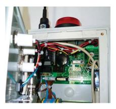
1. Open the PSS Controller door to gain access to the PCB.
